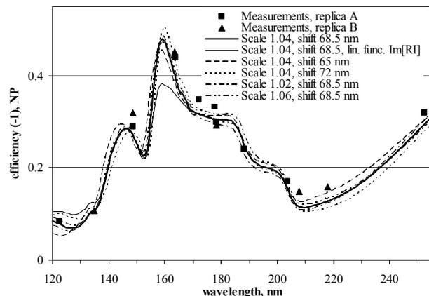
Figure 3. Measured (symbols) and calculated (curves) non-polarized efficiencies of G185M grating plotted vs.  $\lambda$ .
