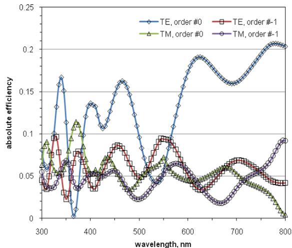
Figure 5. Efficiency of orders of a trapezoidal Si grating with the profile parameters to be reconstructed,  $\theta = 40^\circ$ , plotted vs  $\lambda$ .
