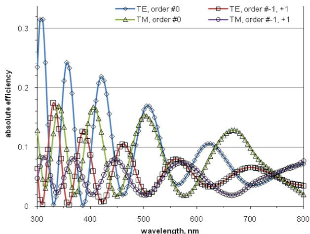
Figure 4. Efficiency of orders of a trapezoidal Si grating with the profile parameters to be reconstructed and  $\theta = 0$ , plotted vs  $\lambda$ .
