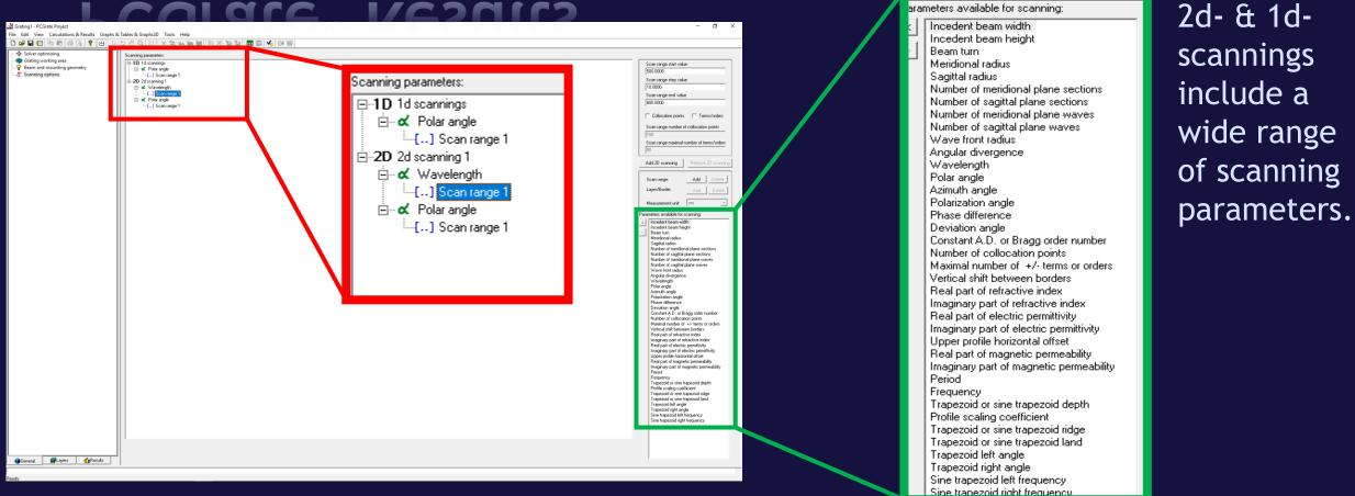
PCGrate<sup>®</sup> includes 2d scanning & 3d efficiency plots. 2d scanning allows one to vary two independent parameters together to solve grating efficiency tasks.
