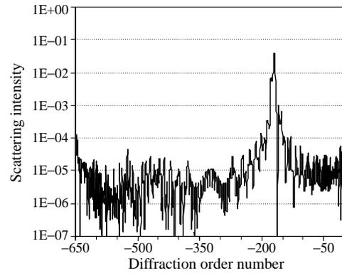
**Fig. 2.** Absolute specular and non-specular reflectivity calculated for sample F667 with vertically correlated GDs at a 0.154-nm wavelength and a  $0.5^\circ$  grazing incidence vs diffraction angle in the range from  $-85.7^\circ$  to  $+89.7^\circ$ . The strong peak exists near a scattering angle of  $28.5^\circ$  that corresponds to specular reflection from QD facets.
