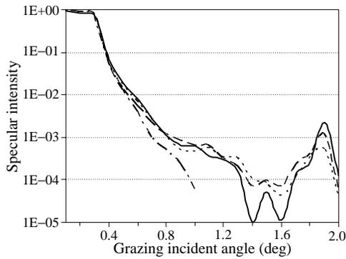
**Fig. 1.** Absolute specular reflectivity for sample F668 with vertically non-correlated GDs at a 0.154-nm wavelength vs grazing angle of incidence: perfect plane structure model (short-dashed line); Névt-Croce approximation with rms roughness of 1.45 nm for triangles (long-dashed line); rigorous calculation with QD height  $h = 5$  nm and width  $L = 16.7$  nm (full line); measurement (long-short-dashed line).
