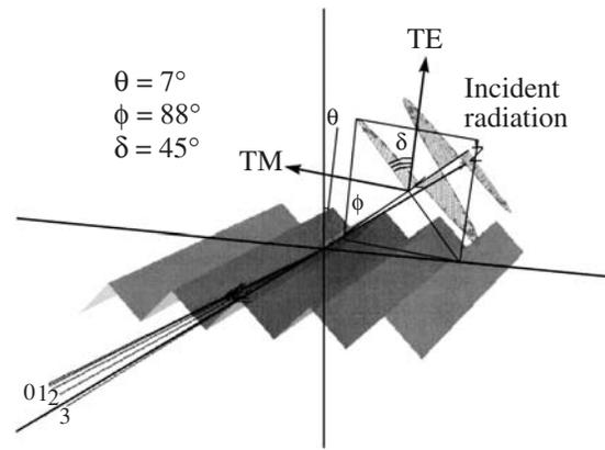
Fig. 1. Schematic representation of the off-plane grating and conical diffraction grazing incidence.
