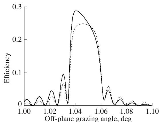
**Fig. 3.** Absolute efficiency of the zeroth (solid curve) and first (dashed curve) diffraction orders of the multilayer (100 Ru/C pairs, 5000 lines/mm) grating with lamellar profile of grooves of depth  $h_1$  and roughness/interdiffusion RMSD of 0.2 nm, calculated for incidence of unpolarized radiation with a wavelength of 0.1 nm at a polar angle of  $0^\circ$ , as a function of the azimuthal grazing angle.
