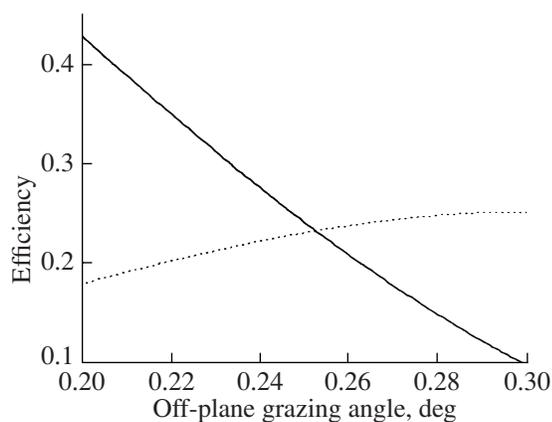
**Fig. 2.** Absolute efficiency of the zeroth (solid curve) and first (dashed curve) diffraction orders of the Pt grating (5000 lines/mm) with the lamellar profile of grooves of depth  $h_0$  and roughness RMSD of 0.2 nm, calculated for incidence of TE polarized radiation with a wavelength of 0.1 nm at a polar angle of  $0^\circ$ , as a function of the azimuthal grazing angle.
