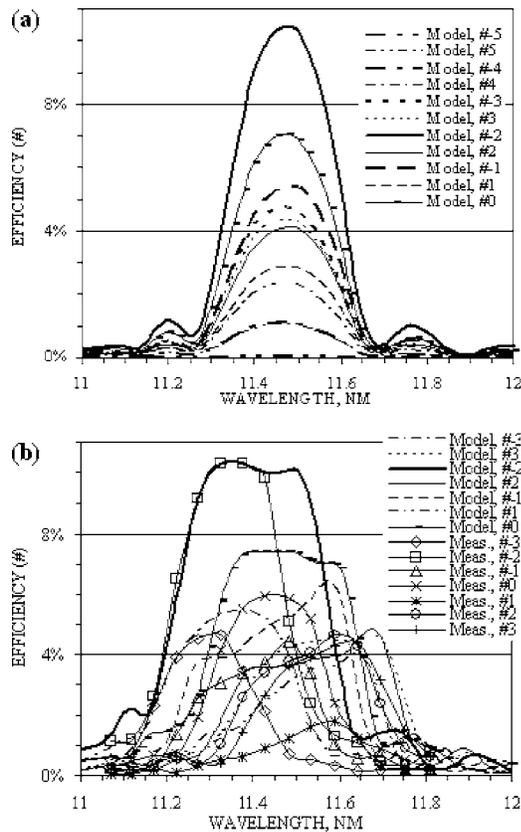
FIG. 7. The measured [(b), curves with markers], approximately calculated (a), and rigorously calculated [(b), curves without markers] efficiencies vs wavelength of the  $-3$  to  $+3$  orders of a 2400-groove/mm multilayer-coated grating with 50 MoRu/Be periods operating at an angle of incidence of  $13.9^\circ$ .
