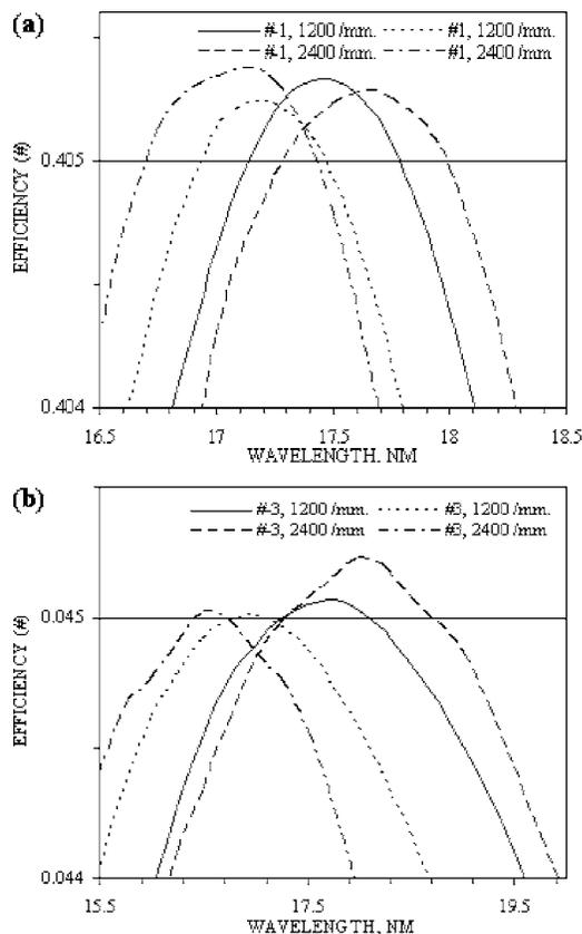
FIG. 4. Rigorously calculated  $\pm 1$  (a) and  $\pm 3$  (b) order efficiencies vs wavelength of perfectly conductive 1200 and 2400-groove/mm lamellar gratings with 5-nm-deep grooves and 0.5 land-to-period ratio operating at an angle of incidence of  $30^\circ$ .
