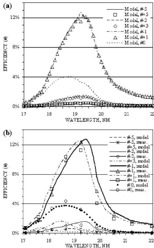
FIG. 8. The measured [(b), data markers], approximately calculated (a), and rigorously calculated [(b) curves] order efficiencies vs wavelength of the 4200-groove/mm multilayer-coated FL1 flight grating, with 20 Mo/Si periods on the short-band side of the EIS optics, operating at an angle of incidence of  $6.5^\circ$ .
