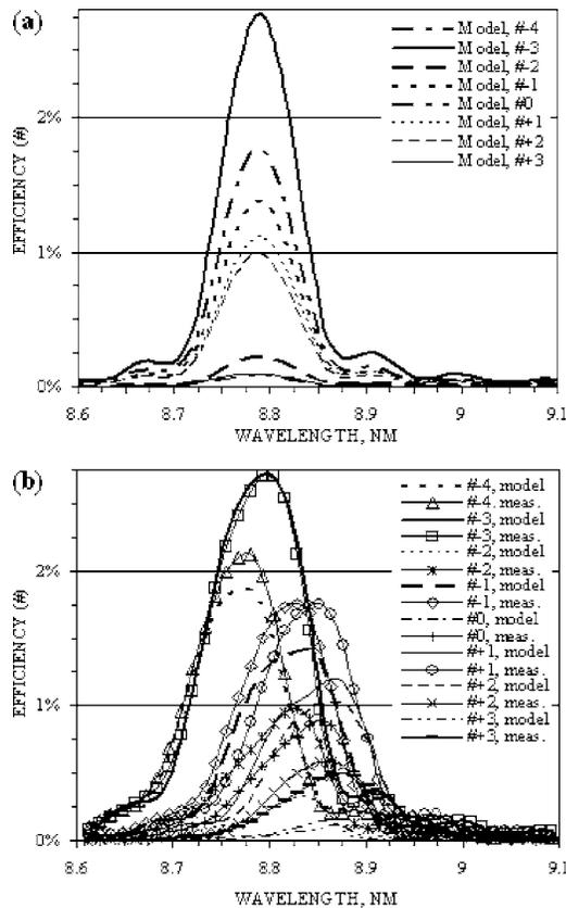
FIG. 9. The measured [(b), curves with markers], approximately calculated (a), and rigorously calculated [(b), curves without markers] efficiencies vs wavelength of the  $-4$  to  $+3$  orders of a multilayer-coated 2400-groove/mm grating with 100 Mo/Y periods operating at an angle of incidence of  $8^\circ$ .
