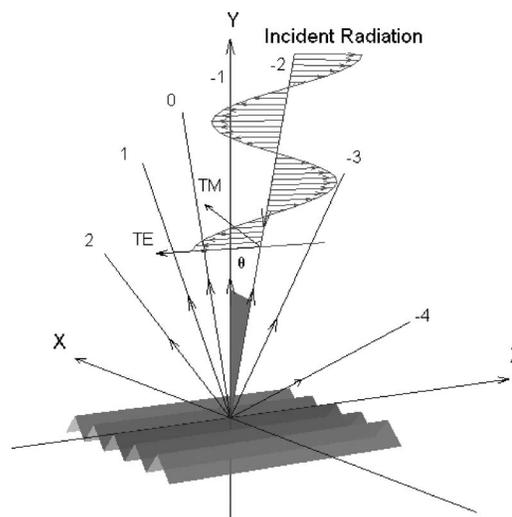
FIG. 2. Light diffraction on a grating working in the autocollimation (Littrow) mounting.
