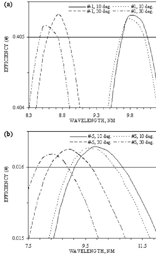
FIG. 3. Rigorously calculated  $\pm 1$  (a) and  $\pm 5$  (b) order efficiencies vs wavelength of perfectly conductive 2400-groove/mm lamellar gratings with 2.5-nm-deep grooves and 0.5 land-to-period ratio operating at angles of incidence of  $10^\circ$  and  $30^\circ$ .
