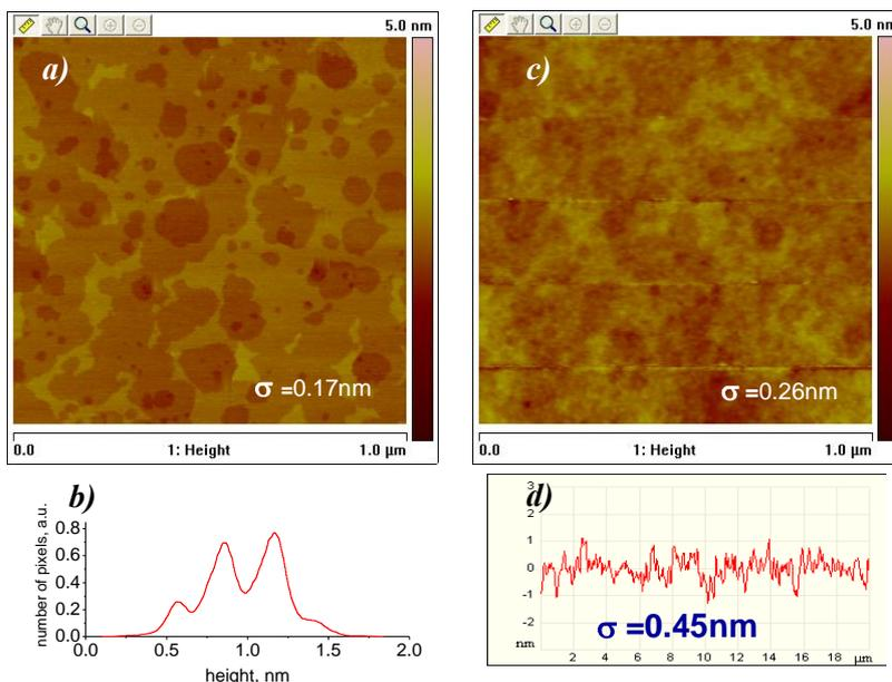
**Figure 1.** An AFM image of a  $1 \times 1 \mu\text{m}^2$  area of anisotropically etched (111) surface of Si (a) and a height distribution in the same area (b); an AFM image of a  $1 \times 1 \mu\text{m}$  area of a saw-tooth substrate with an average groove profile subtracted shows residual high frequency roughness (c), and a  $20 \mu\text{m}$  long AFM scan along a groove of a saw-tooth substrate shows mid-frequency roughness (d).
