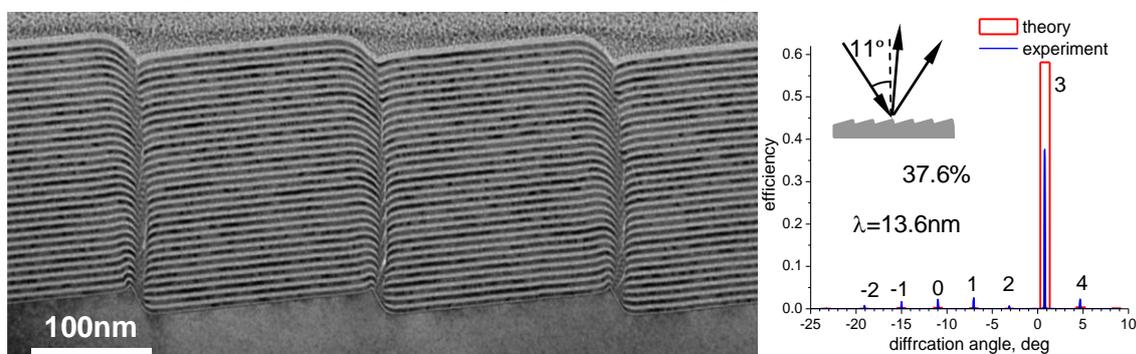
**Figure 2.** Cross-section TEM image of a MBG with groove density of 5000 lines/mm and the blaze angle of  $6^\circ$ , coated with a Mo/Si multilayer (left). Diffraction from the grating at the wavelength of 13.6 nm and the incident angle of  $11^\circ$  (right).
