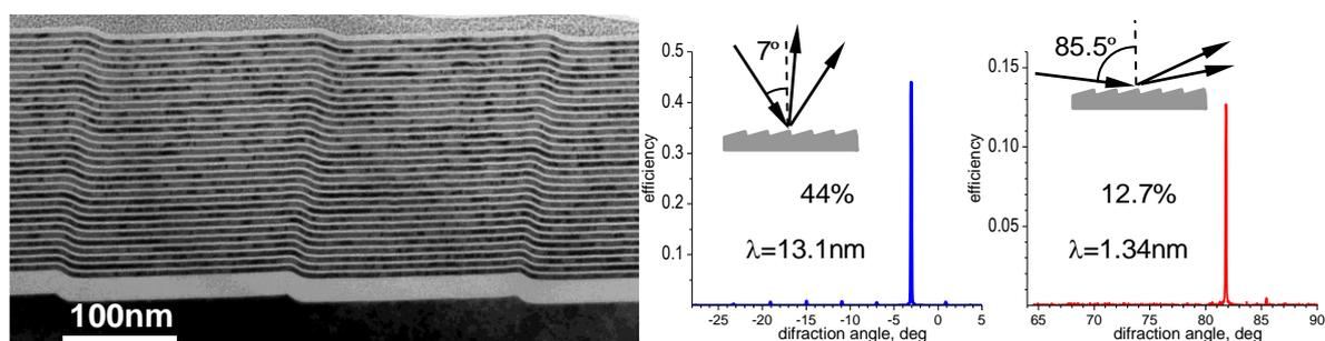
**Figure 3.** Cross-sectional TEM image of a MBG with groove density of 5250 lines/mm and a blaze angle of  $2^\circ$ , coated with a Mo/Si multilayer (left). Diffraction from the grating at the wavelength of 13.1 nm and an incident angle of  $7^\circ$  (center), and 1.34 nm and  $85.5^\circ$  (right).
